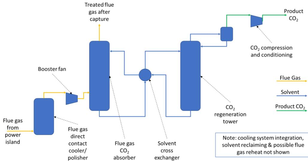
**Figure 1: Post Combustion Carbon Capture Scheme**
