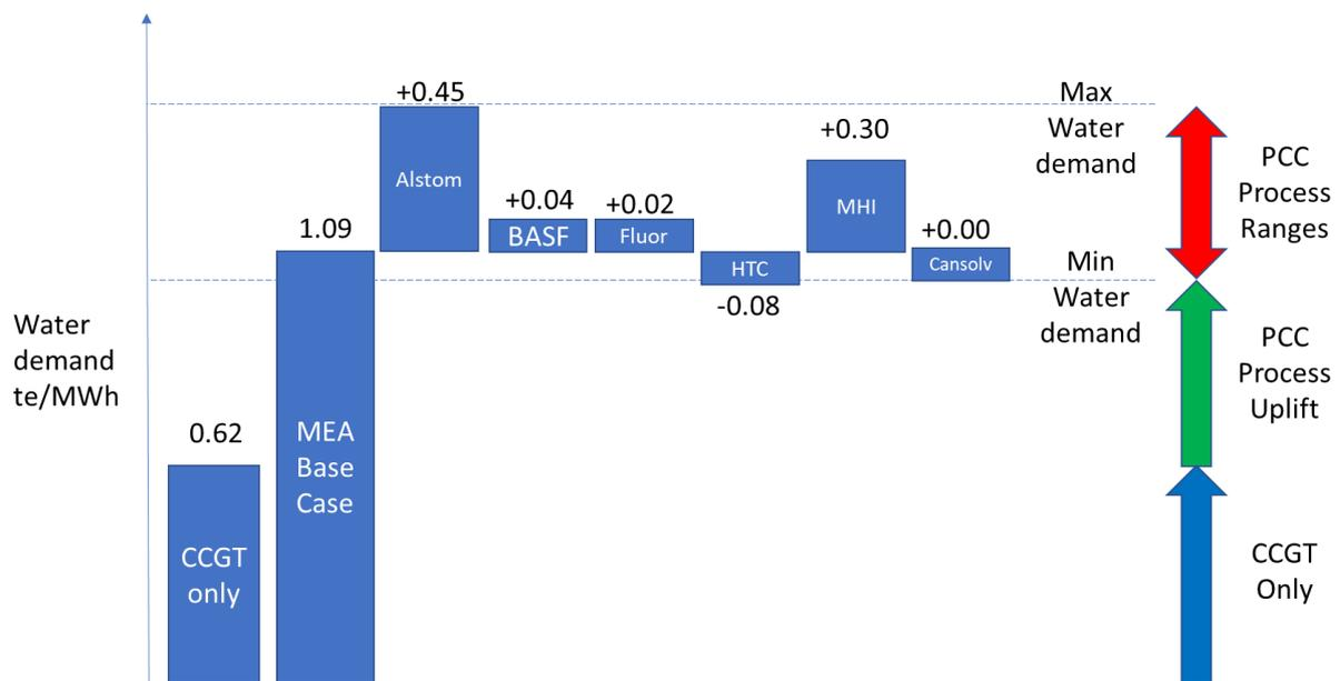
**Figure 3: Total Water Requirement for CCGT+PCC [6]**
